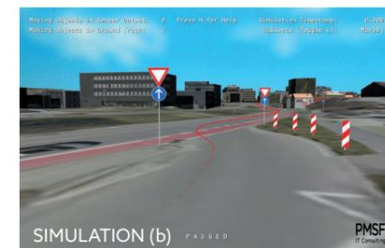
(b) Simulation: Reconstructed test drive. Red dots are the GPS.
